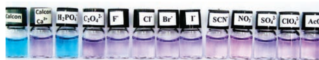
Figure 4. From left to right: calcon (40 \mu M), calcon/Ca 2+ (40 \mu M/120 \mu M) without any additional anion as well as after the addition of either H 2 PO 4 - , C 2 O 4 2- , F - , Cl - , Br - , I - , SCN - , NO 3 - , SO 4 2- , ClO 4 - , or AcO - (2 mM) at pH 12.3 (water/4% MeOH).
